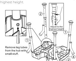
Put tube (a) on (a) in the cross position and then screw tube (b) n B (with parts c (c) in (t) e center. After assembled, turn the cross leg set to opposite side. As shown in partial magnified figure, screw parts (c) & (c) wit leg tube tightly.
