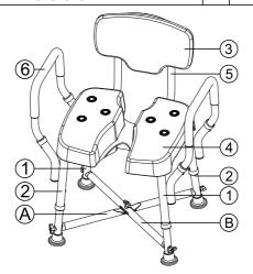
Insert each leg tube 1 & intohe seat 1.2 location. (Caution: For secure installation, make sure the button on each leg is fully engaged to the hub on the seat). Depress the push button and pull the lower leg to the
