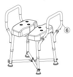
4 Assemble the backrest into back tubes. Fix the four points of tubes 5 onto seat with parts 6 & (caution : for secure installation, make sure the button on each tube is fully engaged to the hub on the
