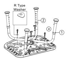
Assemble hand rest into seat and screw it with part (a).
